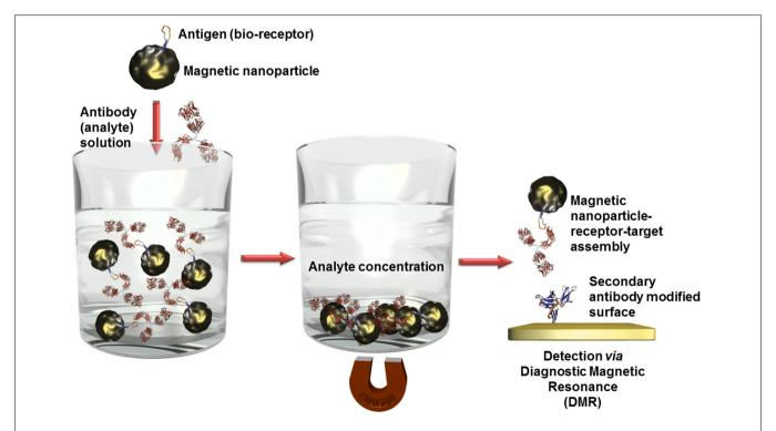
FIGURE 6 | Scheme of analyte concentration in complex solutions via bioreceptor modified magnetic nanoparticles. After the recognition event, the captured analytes can be isolated by precipitation of the magnetic nanoparticles in an external magnetic field. When this magnetic field is
