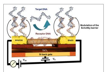
FIGURE 8 | Principle of the modulation of the Schottky barrier at source and drain electrodes of CNT field effect transistor devices after hybridization of the receptor DNA with the target DNA. Here, the wrapping properties of DNA around nanotubes inhibit the capability of this receptor DNA to hybridize with its counterpart and thus deactivate indirectly the CNT channel which remains unaffected toward the recognition event.
