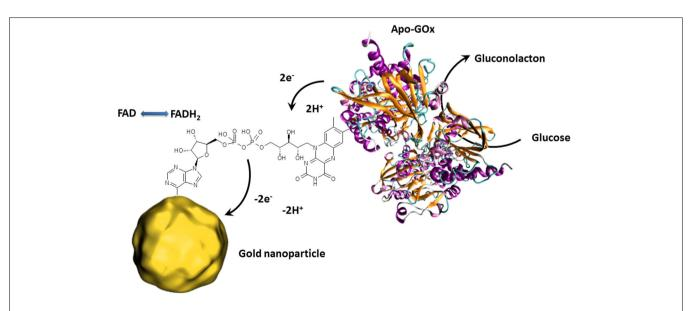
FIGURE 3 | Schematic presentation of the reconstitution of apo-GOx with FAD modified gold nanoparticles enabling the transfer of electron released by the electrocatalytic oxidation of glucose. The collected electrons are then directly transferred to the external circuit giving an electrochemical signal.
