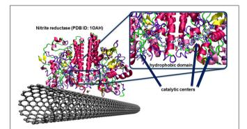
FIGURE 7 | Oriented immobilization of nitrite reductase from Desulfovibrio desulfuricans on CNTs via hydrophobic interactions between the enzyme and the carbon nanotube surface. This naturally occurring adsorption leads to an efficient electron transfer between the enzyme and the conducting surface where the redox center, after catalytic reduction of nitrite ions to ammonia, can directly be regenerated by the electrode.
