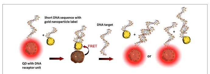
FIGURE 4 | Illustration of the FRET principle between QDs and gold nanoparticles and the reestablishing of fluorescence after the recognition event. The target DNA can hybridize either with the receptor
