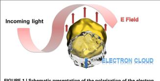
FIGURE 1 | Schematic presentation of the polarization of the electron density at resonant excitation wavelength. At particle sizes smaller than the excitation wavelength, the oscillating electrons (surface plasmons) cannot propagate along the gold surface leading to a polarization of the electron cloud at one side of the particle.
