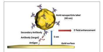
FIGURE 2 | Illustration of the perturbation of propagating surface plasmons on gold surfaces provoked by gold nanoparticles of defined size and distance leading to an additional change of the evanescent field and therefore to an enhanced signal.
