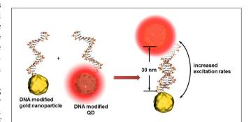
FIGURE 5 | Principle of the antenna effect of gold nanoparticles enhancing the excitation rates of QDs when positioned at  $\sim$ 30 nm.
